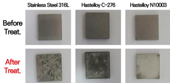
Fig.2. Naked eye vision image of before/after corrosion immersion test
