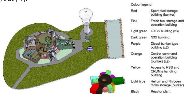
Fig. 1. General design of a GFR plant layout [2] (HSS = Helium Supply Service; GTCS = Gas Turbine Conversion System; N3S = Nuclear Steam Supply System; CRDM = Control Rod Drive Mechanism)
