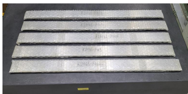
Fig. 1. Images of 5.3 \text{ gU/cm}^3 of high-density U_3Si_2 dispersion fuel plates for irradiation test.
