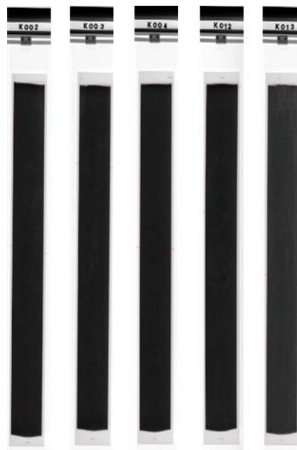
Fig. 2. Radiographic test images of 5.3 \text{ gU/cm}^3 of high-density U_3Si_2 dispersion fuel plates for irradiation test.
