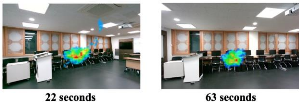
Fig. 2. Real-time contextual data updated radiation images projected on RGB images of the ^{137}\text{Cs} source at 22 and 63 seconds.
