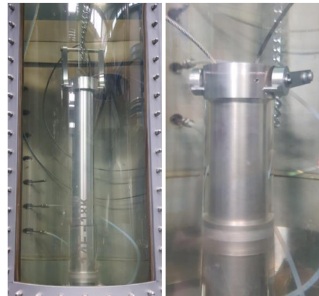
Fig. 3. Out-of-reactor test for cobalt SPND HANARO test
