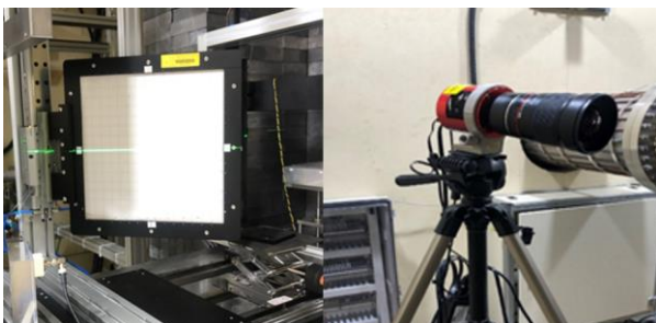
Fig. 1. Setup of the P43 phosphor screen and TE-cooled CMOS camera at TR103
