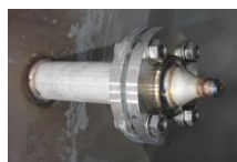
(c) Horizontal injection nozzle
