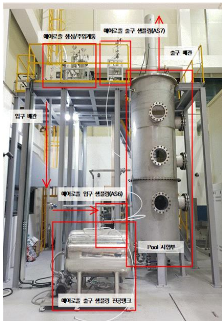
Fig 3. Picture of aerosol pool scrubbing facility
