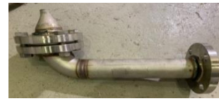
(d) Vertical orientation of injection nozzle Fig 4. Configuration of injection nozzle
