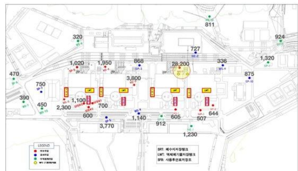
Fig. 2. Groundwater monitoring wells and maximum concentration of tritium on May 2019 at Wolsong NPPs (unit: Bq/L).
