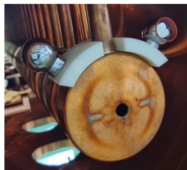
Fig. 3. New type jig to measure DT coordinate
