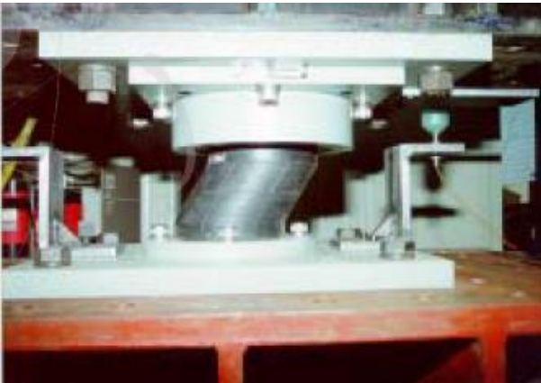
Fig. 4 Shear-Compression Test for 3D-LRB
