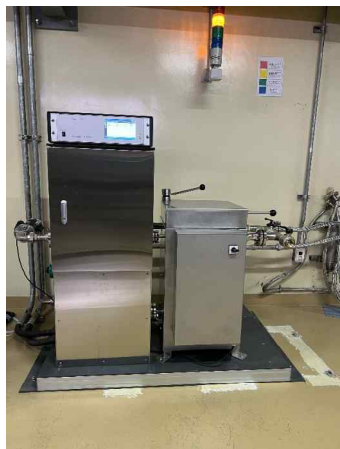
Fig. 1. Liquid monitoring system using a NaI(Tl) detector
