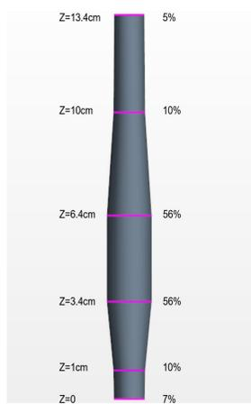
Fig. 2 The strained cladding in 192 model
