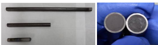
Fig. 1. Fabricated simulated damaged spent fuel rodcuts (left)
