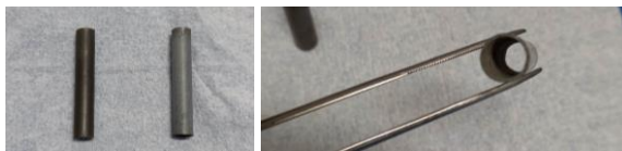
Fig. 4. Comparison of 5cm rodcuts before and after oxidation test (left) and completely decaldded hull (right)
