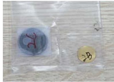
Fig. 1. The Cd covered Au foil sample (left) and bare Au foil sample (right)
