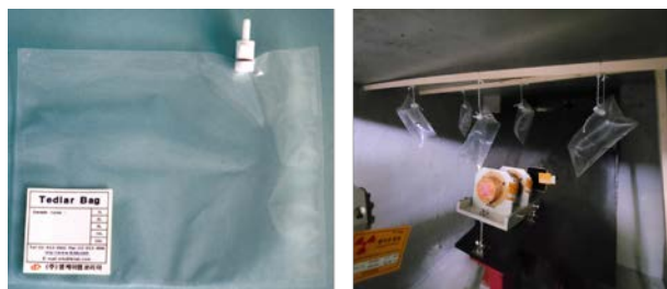
Fig. 3. Sampling bag for ^{40}\text{Ar} gas (left) and sample installation around the electron beam dump (right)
