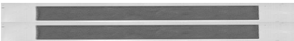
Fig. 4. UT images of foreign bodies injected high density U 3 Si 2 fuel plates
