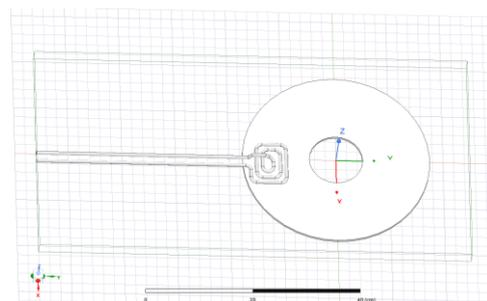
Fig. 2. Simplified geometry of graphite target, and copper coil
