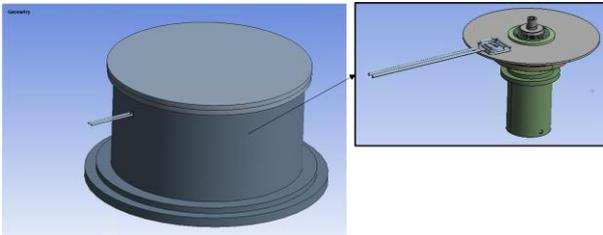
Fig. 3. Chamber geometry (Left) Graphite target, copper coil, and detailed parts (Right)
