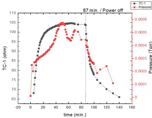
Fig. 4. Measured thermocouple resistance per minute (Black) Internal pressure in vacuum chamber (Red)
