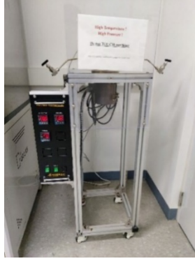
Fig. 1. Static autoclave corrosion test apparatus.
