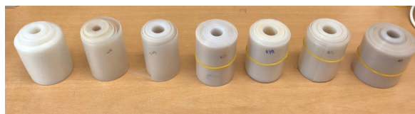
Fig 1. Fabricated boehmite/HDPE nanocomposite films containing nanoparticles coated with various modifiers.
