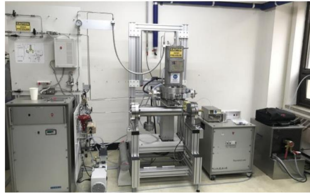
Fig. 1. High pressure steam environment STA
