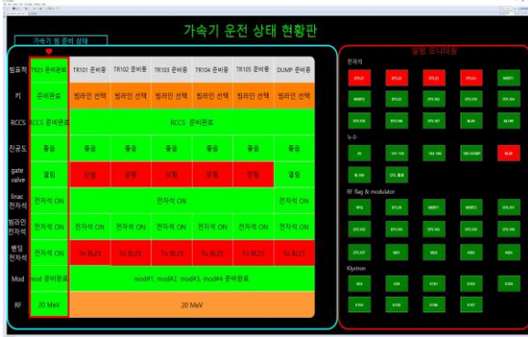
Fig. 3. LINAC status monitoring system for KOMAC
