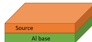
Fig. 4: Input geometry. Surface area is 10x10 cm, the backing aluminum base has 0.01 cm. Source thickness varied.
