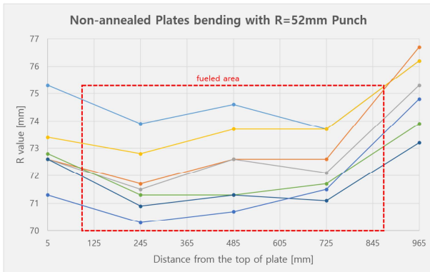
Fig. 2. Plate-forming results of non-annealed fuel plates
