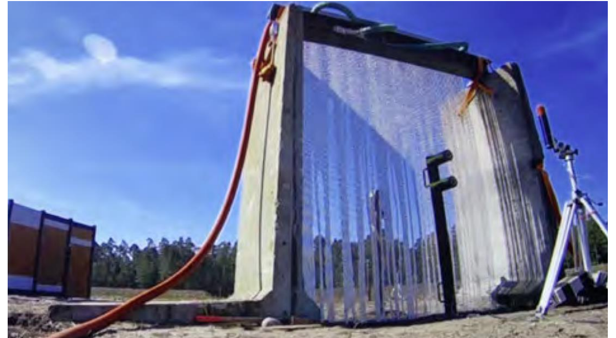
Chain & Water Curtain: Reduction of Pressure Wave up to 50%
