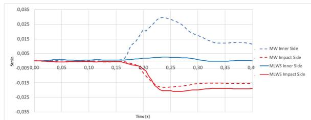
Fig. 9. Maximum tension and compression strain of MW and MLWS
