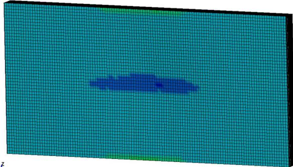
Fig. 6. MLWS max. Compression Strain on Impacted Side 2,10 %
