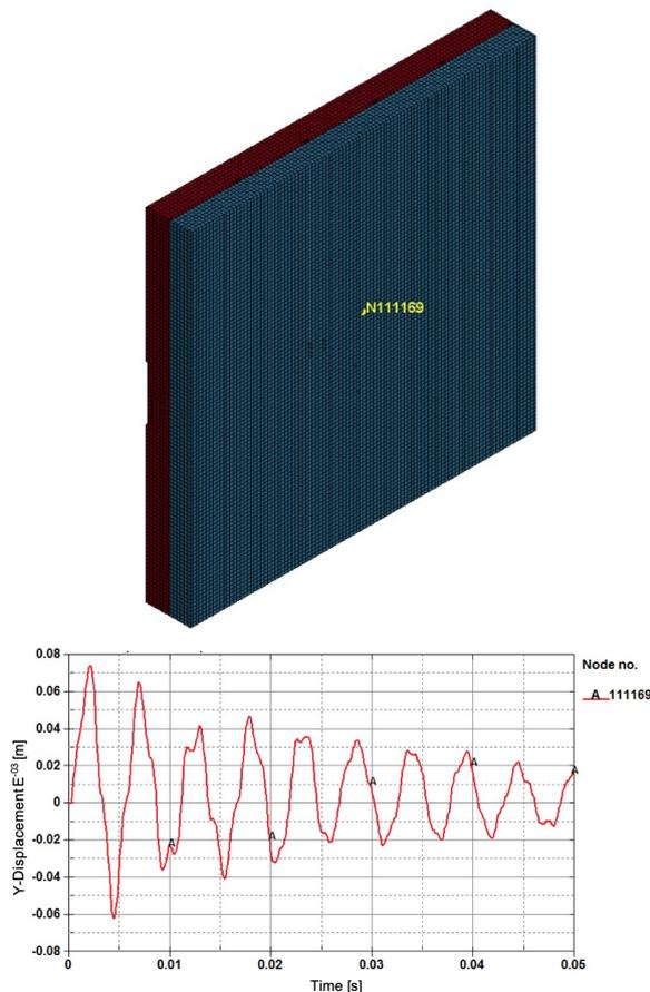
Fig. 21. Dynamic Response of the MLWS at the Inner Side
