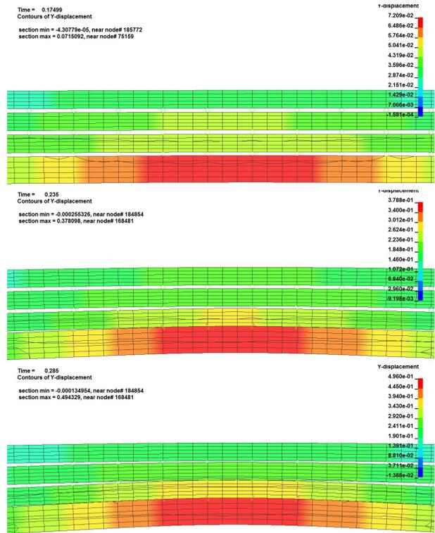
Fig. 8. Deformation states of the Multilayer Wall System due to APC A320
