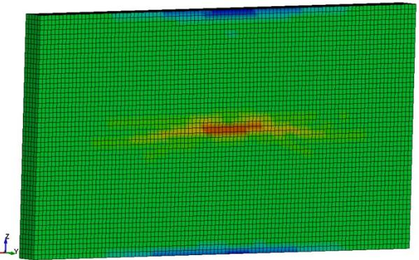
Fig. 3. MW max. Tension Strain on Inner Side: 2.99 %
