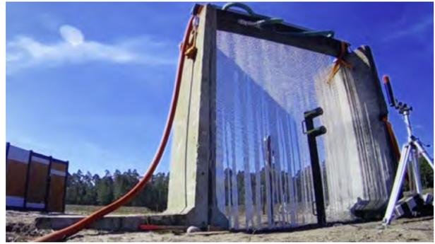
Fig. 11. Chain & Water Curtain: Reduction of Pressure Wave up to 50%
