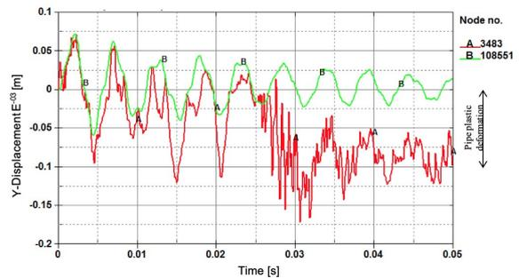
Fig. 20. Dynamic Response of the MLWS at the Inner Side
