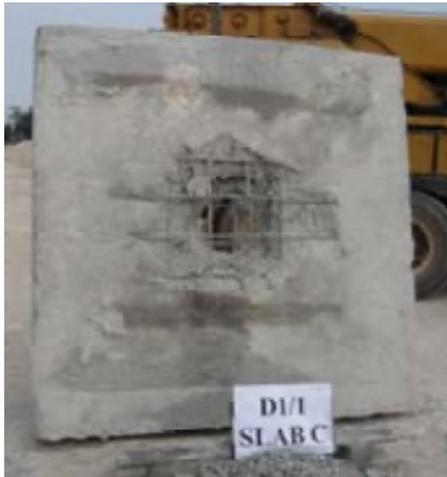
Fig. 12. Damage Pattern of a 30 cm Massive Wall Exposed to 2 kg TNT [14]
