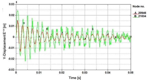
Fig. 17. Dynamic Response of the MW at the Inner Side
