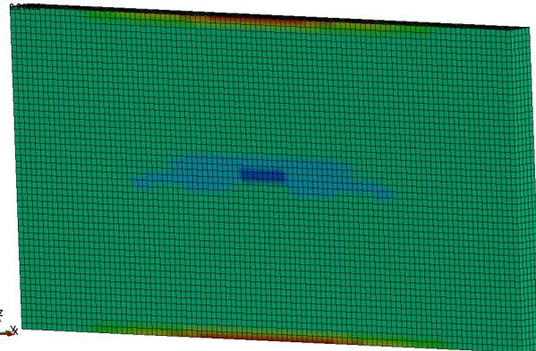
Fig. 2. MW max. Compression Strain on Impact Side: 1,81 %
