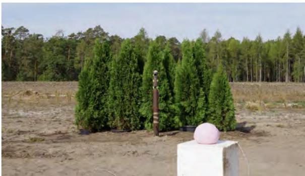
Fig. 10. Green Hedge - Reduction of Pressure Wave up to 60%
