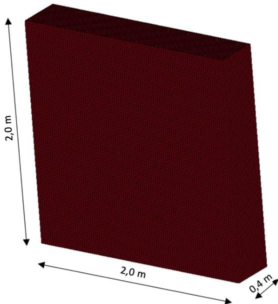
Fig. 13. Finite Element Model of MW
