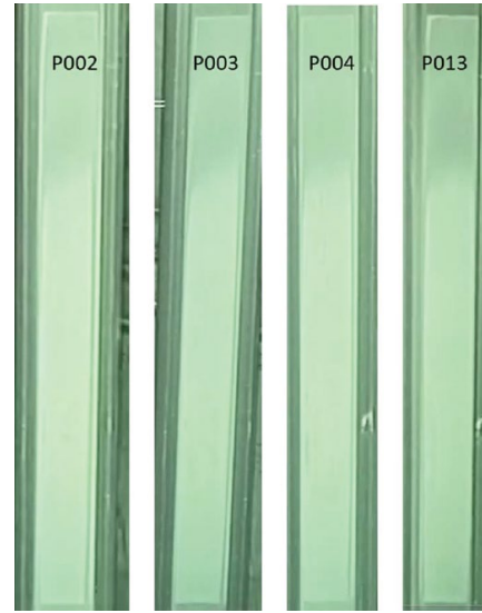
Fig. 4. Visual images of irradiated fuels after 1 st Cycle
