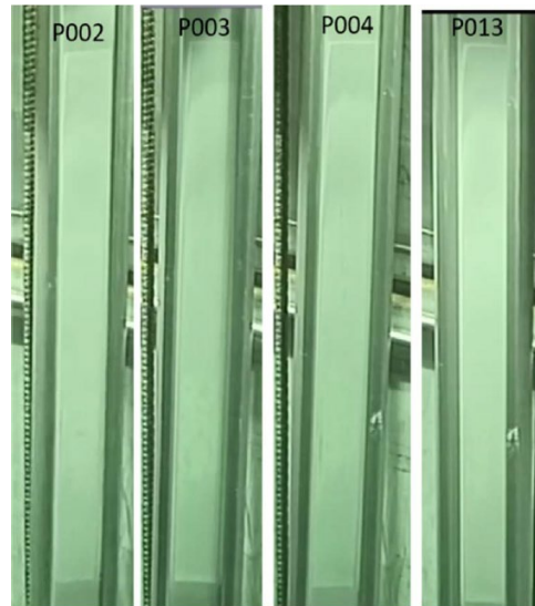
Fig. 5. Visual images of irradiated fuels after 2 nd Cycle
