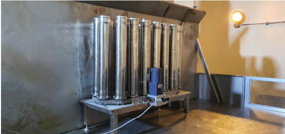
Fig. 2 To evenly irradiate the solidified waste with radiation, a separate rotating device was manufactured and worked.
