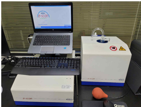
Fig. 3 e-SCAN radiation dose measuring instrument. - An instrument for measuring radiation dose using an alanine dosimeter.
