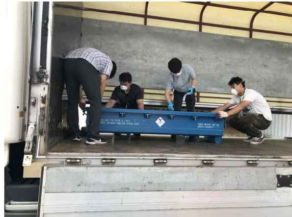
Fig. 4 Packages for transportation to transport solidified waste - unloading radioactive waste.
