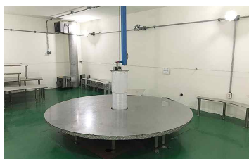
Fig.1 Inside of the low-level irradiation facility - To the central chimney, six radiation sources are climbed from the storage box under the shelf.
