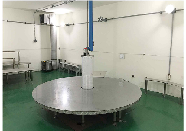
Fig. 1 Inside of the low-level irradiation facility - To the central chimney, six radiation sources are climbed from the storage box under the shelf.
