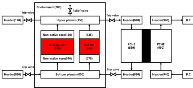
Fig 4. MARS Simulation Node Structure
