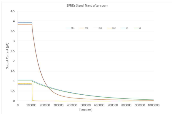
Fig. 3 SPND output signal response after reactor trip
