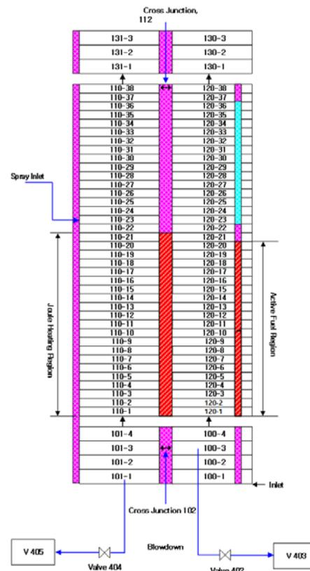
Fig. 2. Nodalization of Halden IFA-650.9 test rig in FAMILY code
