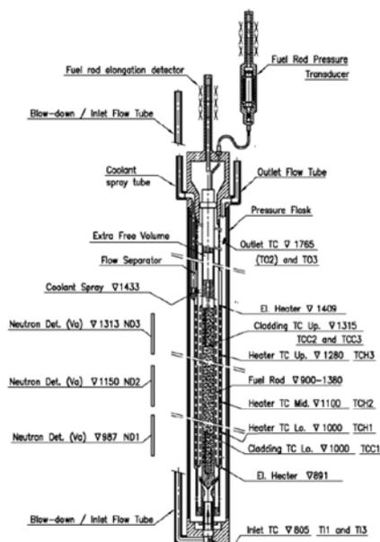
Fig. 1. A schematic of Halden IFA-650.9 test rig
