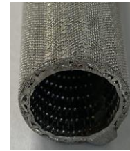
Fig. 3. Configuration of 5-layer sintered wick
