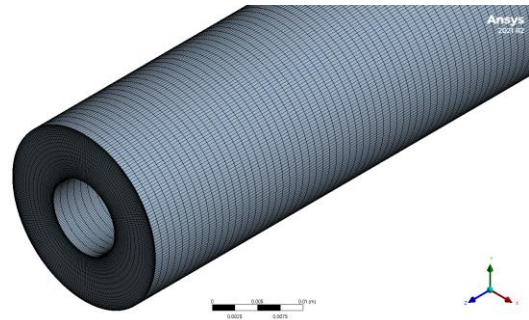
Fig. 4 Mesh of the chimney channel in the DISNY test section
