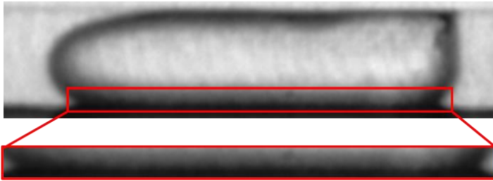
Figure 6. Visualization of Flow Boiling Using Visible Light in this Study Group
