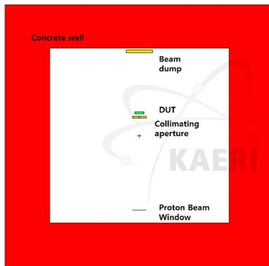
Fig. 4. the calculation model of MCNPX code
