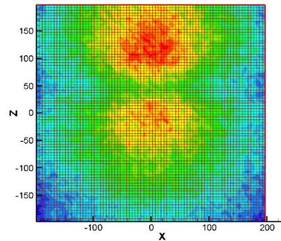
Fig. 6. the spatial distribution of secondary neutrons in the TR102 facility with the collimator
