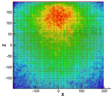
Fig. 5. the spatial distribution of secondary neutrons in the TR102 facility without the collimator
