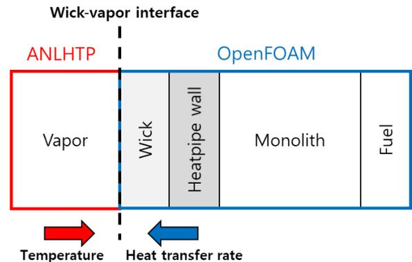
Fig. 1. Data exchange strategy at the wick-vapor interface of heat pipe for the OpenFOAM-ANLHTP code coupling
