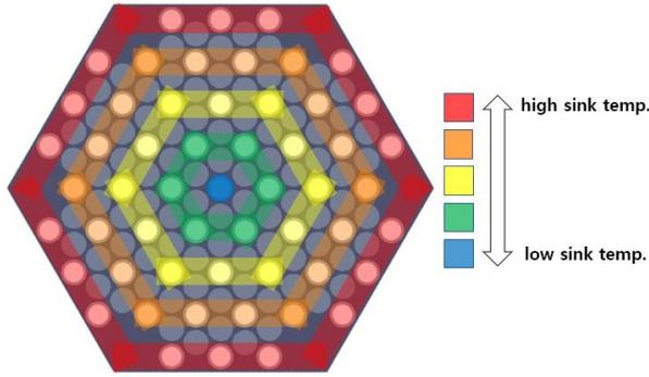
Fig. 5. Heat pipe grouping for adjusting heat sink temperature
