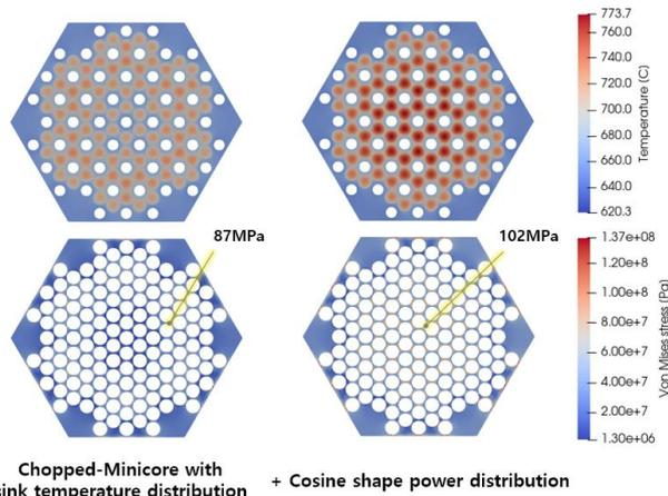
Fig. 6. Thermal-structural analysis of the chopped-Minicores with different heat pipe sink temperature and power distribution
