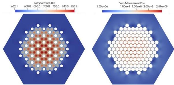
Fig. 3. Thermal-structural analysis results of the Minicore
