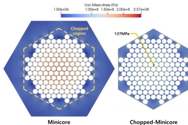
Fig. 4. Comparison of the structural analysis result of the Minicore and the chopped-Minicore
