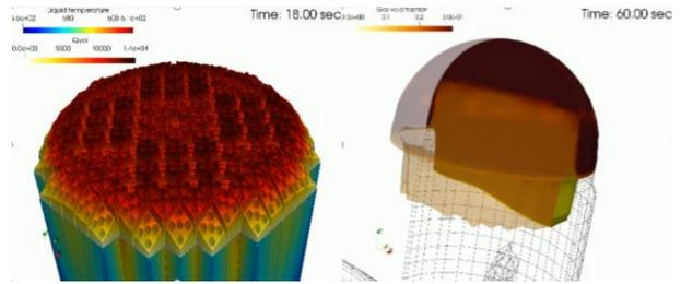
Fig. 5. Key phenomena in the RPV during SLB accident: Left – Overpower distribution prior to setpoint, Right – Occurrence of void fraction in upper head
