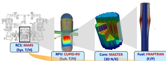
Fig. 1. System configuration for MSMP
