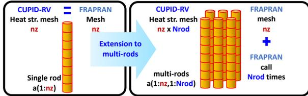
Fig. 3. Schematics of multi-rod extension in CUPID-FRAPTRAN coupling
