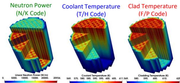
Fig. 4. Verification of CUPID/MASTER/FRAPTRAN Coupled code – Steady state of OPR1000
