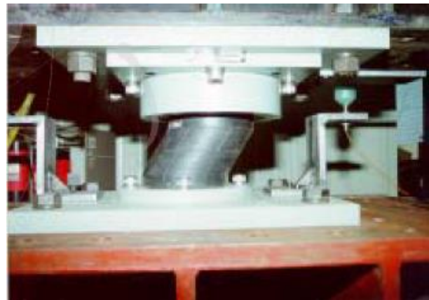
Fig. 1 Shear-Compression Test for 3D-LRB
