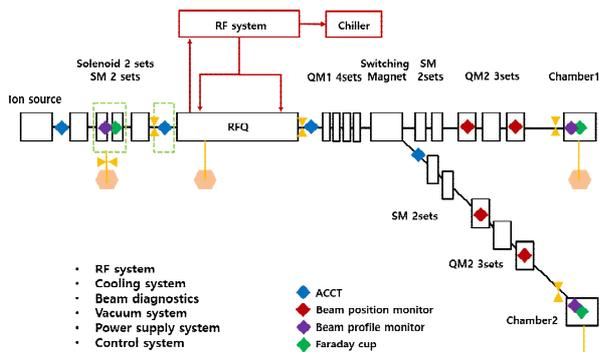
Fig. 1. Layout of 1 MeV/n RFQ machine
