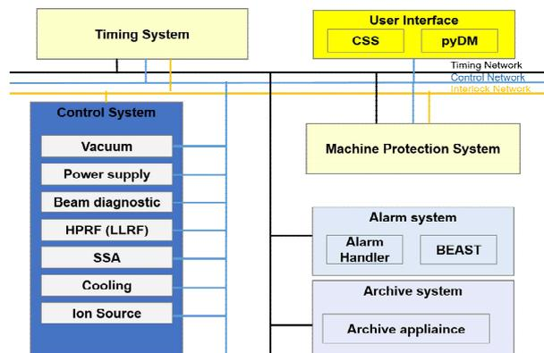
Fig. 2. Layout of EPICS based Control System
