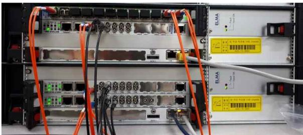
Fig. 4. Event timing system for timing distribution
