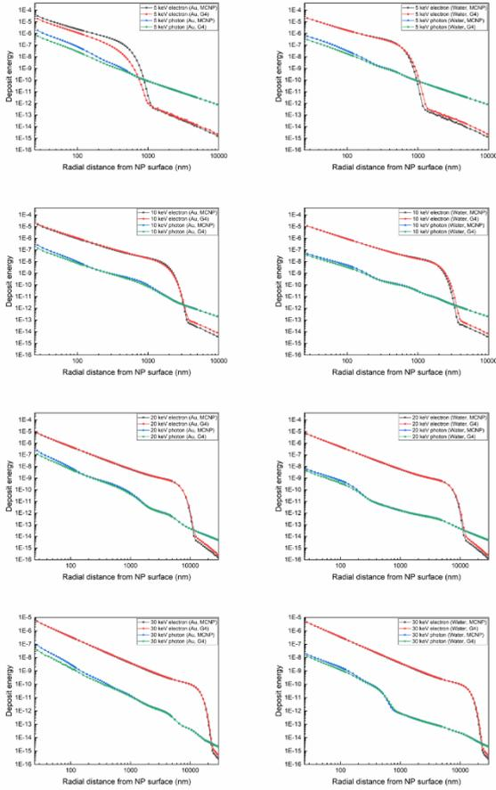
Fig. 2. Radial energy deposition along the radial distance from the surface of GNP. The left rows show the radial energy deposition with gold nanoshell, and the right rows show the radial energy deposition with water nanoshell.
