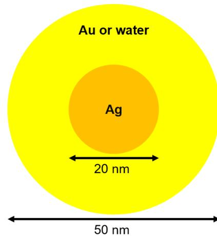
Fig. 1. Illustration of MC simulation geometry in MCNP6.2 and Geant4.
