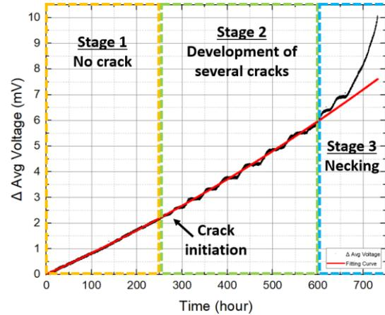
Fig. 2. Detection method of crack initiating moment by interpreting direct current potential drop data
