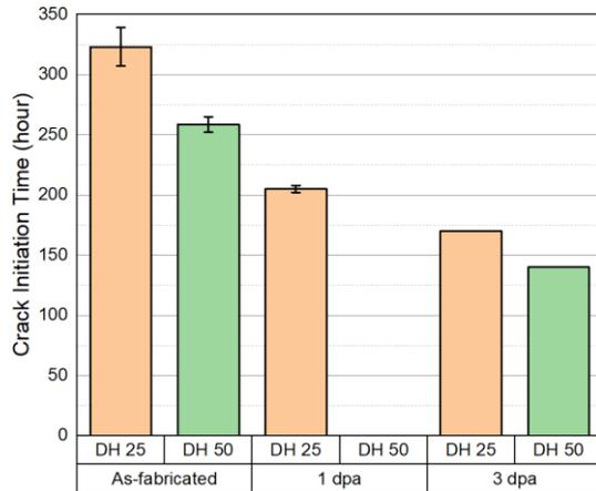
Fig. 3. Summary of crack initiation time measurement with differing the amount of radiation damage and dissolved hydrogen concentration
