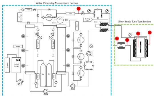
Fig. 1. Schematic diagram of experimental facility which consists of water chemistry maintenance section and stress corrosion cracking experimental section
