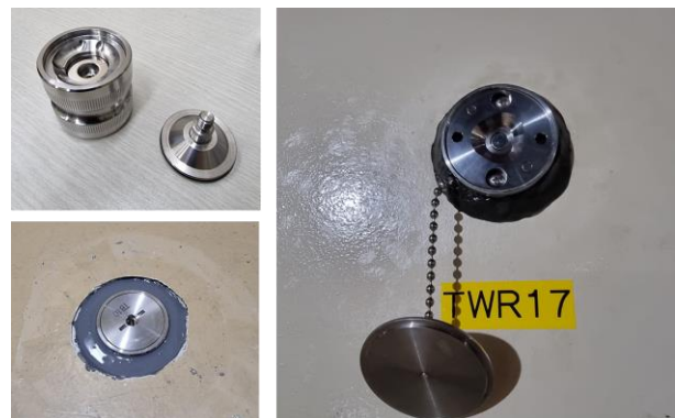
Fig. 2. Reflector mount for the floor(left) and the wall(right)
