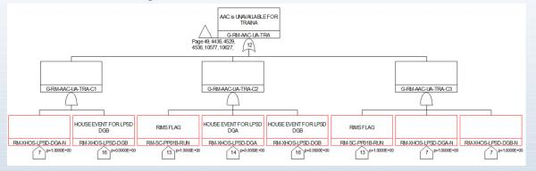
To implement the principles above, 4.16kV train Bravo has the flag combination logic below.
