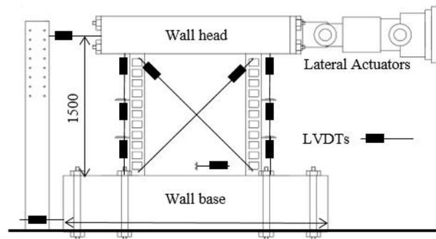
Figure. 1. Test set up
