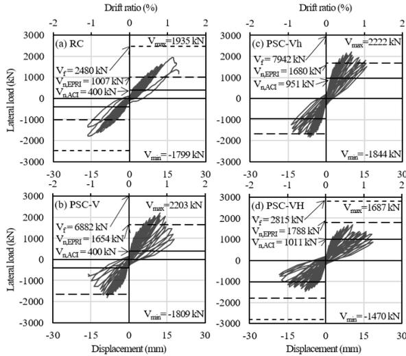
Figure 2. Lateral load-displacement relationship of specimens.
