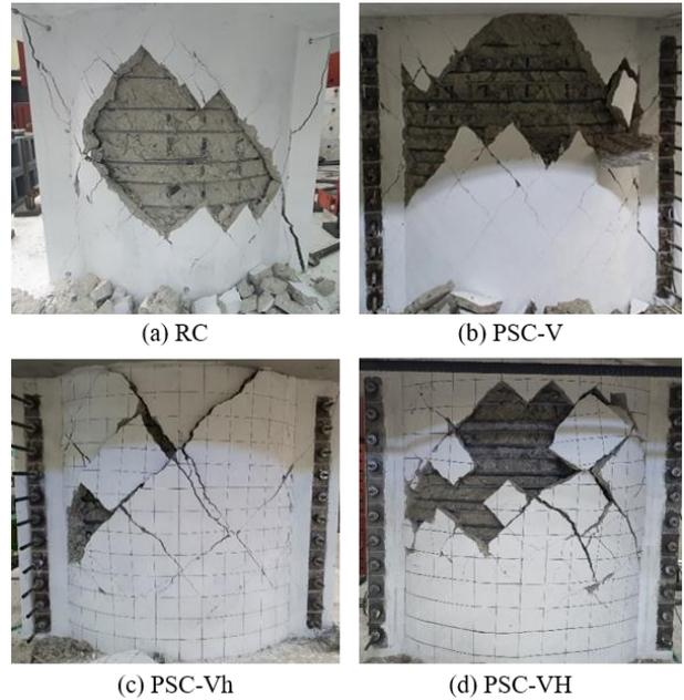
Figure 3. Failure mode of cylindrical wall
