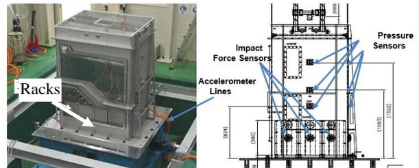
Fig. 1. One-eighth model of a SFSP and racks
