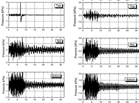
Fig. 3. Dynamic pressure measurements on the walls of SFSP at 0.2g (three left column) and 0.3g (three right column) seismic input.
