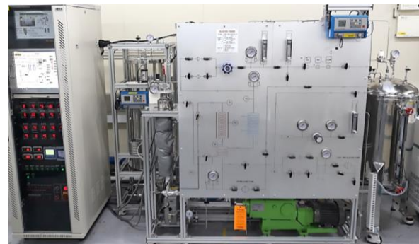
Fig. 1. Recirculation secondary loop system for SG tube fouling test developed in KAERI.
