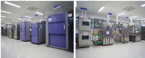
(c) High/low temperature, humidity, low pressure (altitude), temperature shock, salt spray, waterproof and dustproof test, etc
