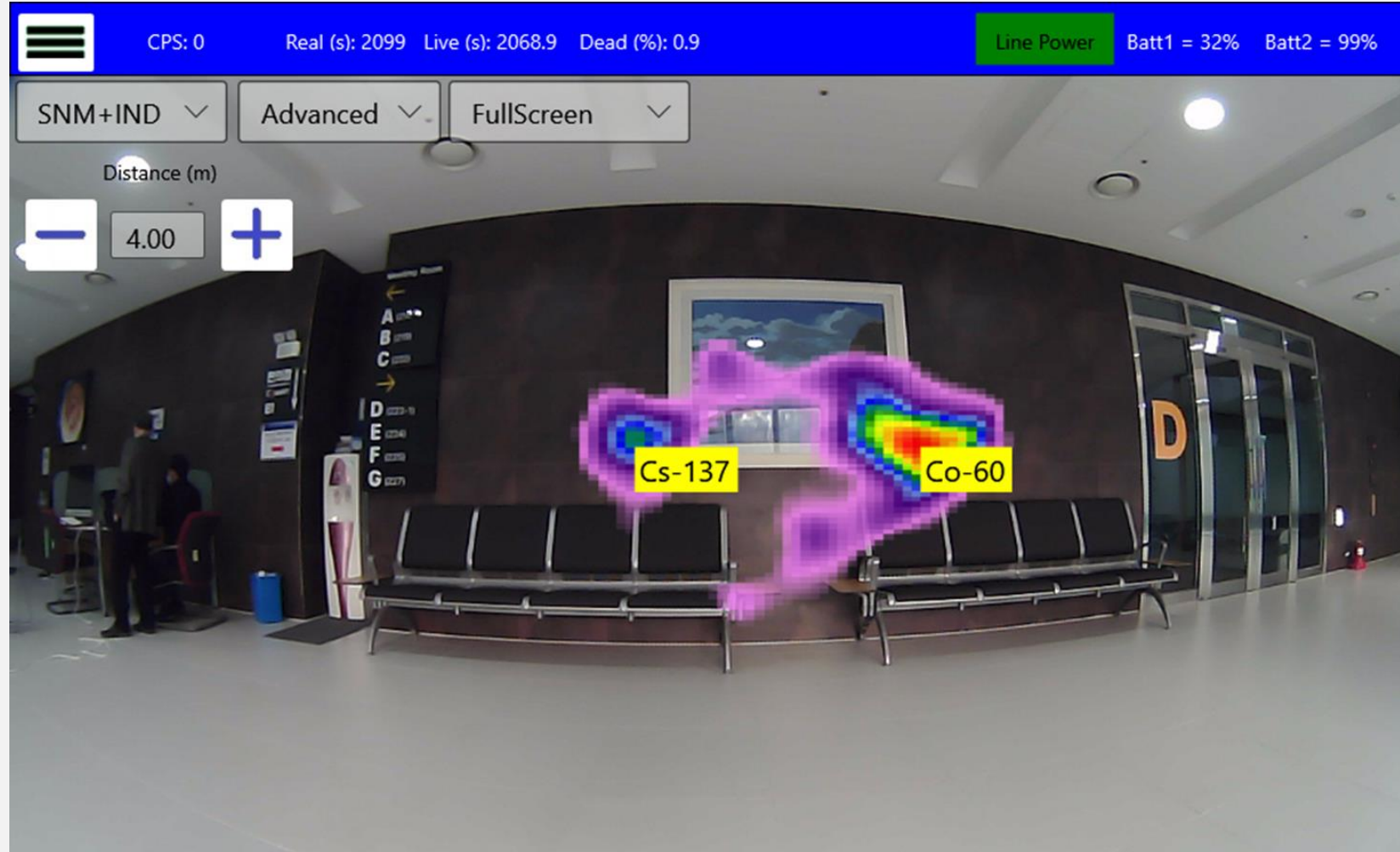
Fig. 3. Compton image by a gamma-ray imager of PHDS Co.
