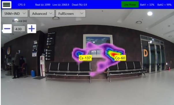
Fig. 3. Source locations and nuclide identification results for the two sources.
