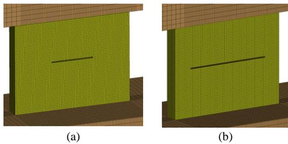
Fig. 4. Concrete voids in shear wall model for (a) 20%, (b) 40% of shear area.
