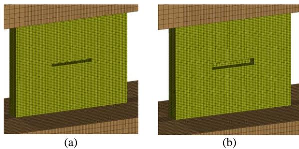
Fig. 5. Concrete voids in shear wall with thickness of (a) 4 cm, (b) 8 cm.
