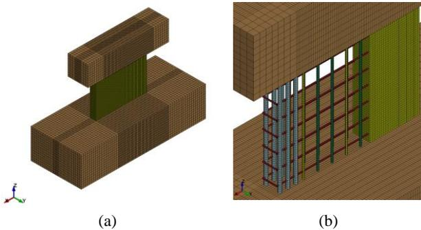
Fig. 3. Numerical models of (a) shear wall and (b) rebar in concrete wall
