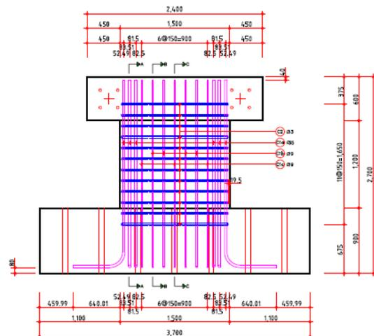
Fig. 2. Reinforcement diagram for shear wall
