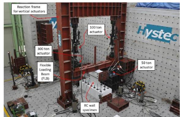
Fig. 1. Shear wall test specimen and experimental setup
